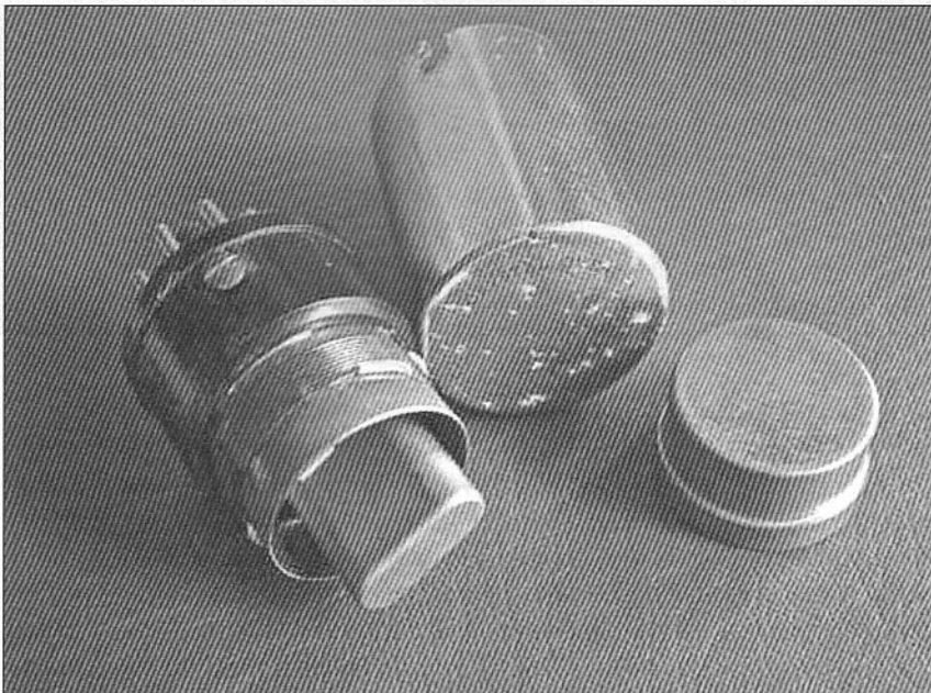
Fig 13.27: Cathodeon crystal oven for HC6/U crystals
