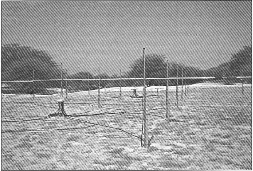
Fig 12.10: Buckland Park VHF meteor radar antenna system
