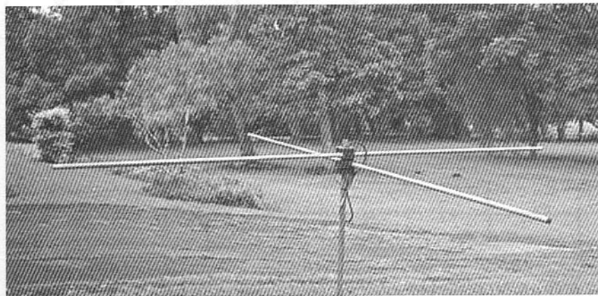
Fig 4.37: Crossed-dipole array for 70 MHz
